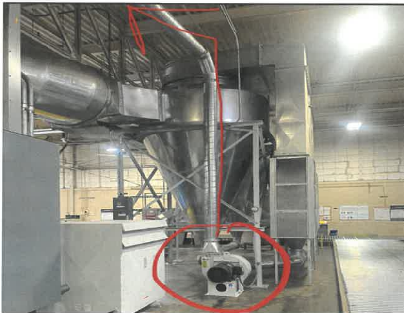
Figure 6: Cyclone fines to connection with the CBP #45 blower that connects to the 18 inch duct that emits to the cyclone on the roof. Cyclone after filters shown just to the right of Twin Cyclones
